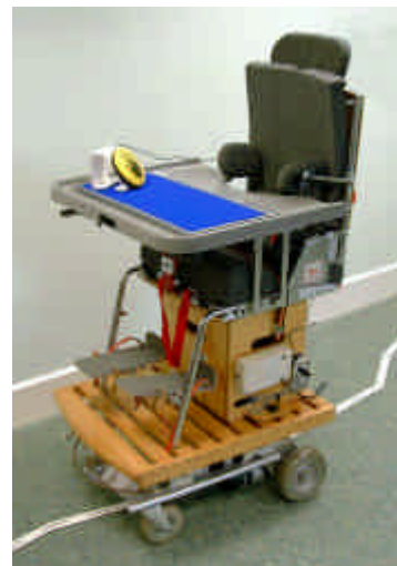
The Big Buddy Button switch angled to enable the user to 'drive' the pre-programmed Mobility Platform
