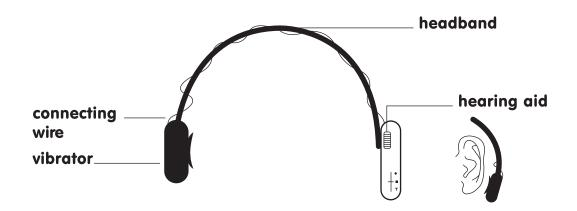
Bone conduction hearing aids work in a different way from other hearing aids. Instead of making sounds louder they change them into vibrations. The vibrations then pass through the bone in the child's head to the cochlea. The vibrations are then converted into sound in the usual way.
