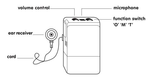
Body worn hearing aids are designed to be worn on the chest. Children who use body worn aids often wear a special chest harness. These harnesses are designed to place the microphone in the correct position and to limit movement of the aid. This can help to reduce unwanted noise.
